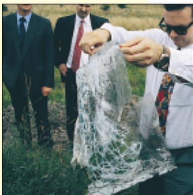
**Glass with film applied is blown out of frame. Fragment hazard greatly reduced. However risk of body impact and loss of controlled environment.**
